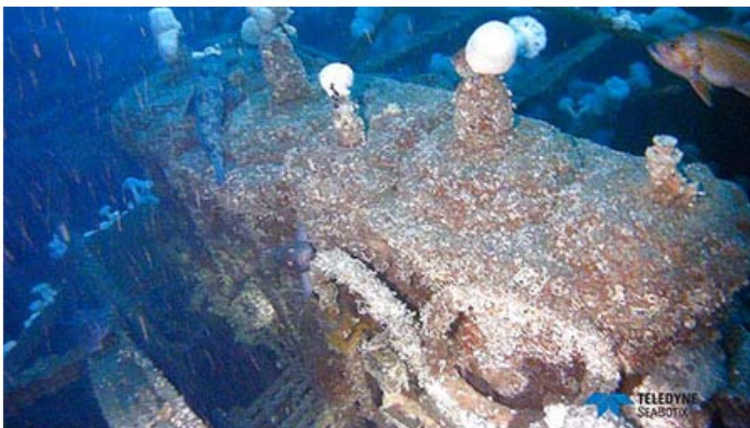
*Figure 8. The triple expansion steam engine built for the steam yacht Ituna by A. & J. Inglis in 1886 in Glasgow, Scotland. Credit: NOAA-Teledyne Seabotix.*
