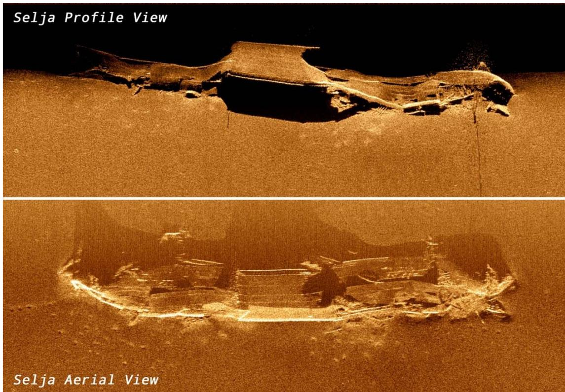
*Figure 11. SS Selja side scan sonar images. Credit: NOAA-Teledyne Seabotix.*
