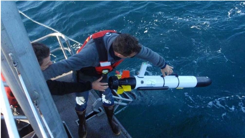
*Figure 4. Teledyne Seabotix vLBV300 ROV used during the October 2015 research expedition. Credit: Tricia Dodds.*
