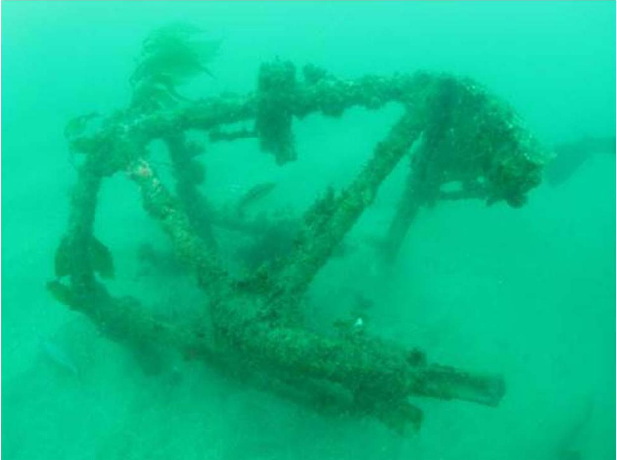
*Figure 12. Forward fuselage of the Corsair, which has been reduced to a skeletal structure.*
