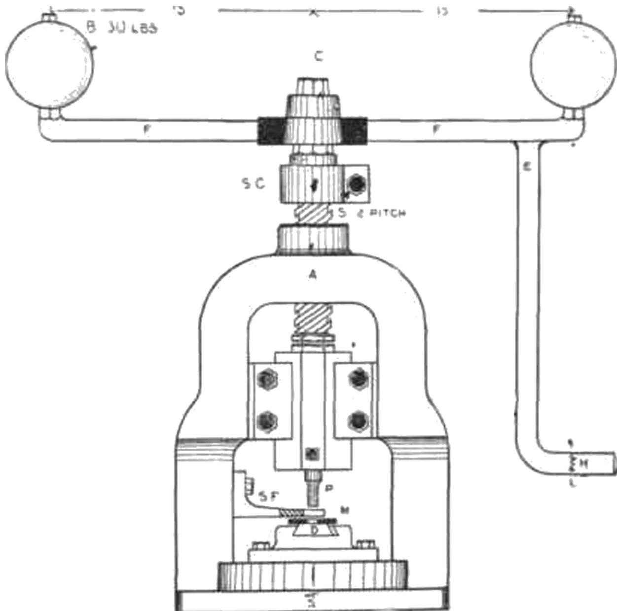
Figure 2. A fly press similar to this one likely was used to produce Prosser beads.
